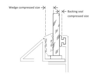
Prior to final assembly, it should be checked that the locating fins on the wedge correctly fit the serrations in the aluminum extrusion. It is important that the wedge is the correct size. An oversized wedge will increase the risk of glass breakage. Likewise, a smaller wedge will eventually fall out and expose the glazing unit to weather damage.
