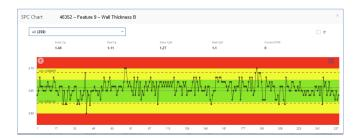
If there is an out of specification measurement (Red zone) the operator is guided to an eTag (non-conformance) recording window, the Production and Quality managers receive an email message.
